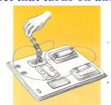
A magnet can be made by winding an insulated wire around an iron core and running current through the wire. The magnetism produced by an electromagnet can be turned on and off using a switch.
