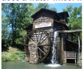
A waterwheel is an axle with blades that are pushed by flowing or falling water. The flow of water is strong enough to make objects move.
